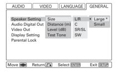
Select the size (Large\* or Small) independently for the L/R (front pair of speakers), the C (center speaker) and the SR/SL (surround pair of speakers). Turn the subwoofer (SW) ON\* or OFF (if you have no subwoofer).
